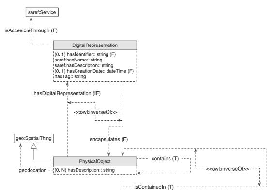
Figure 6: Physical object and digital representation model
