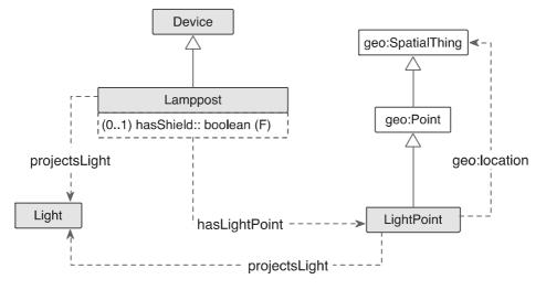
Figure 8: Lamppost and light point model
