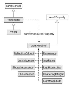
Figure 7: Photometer and light property model
